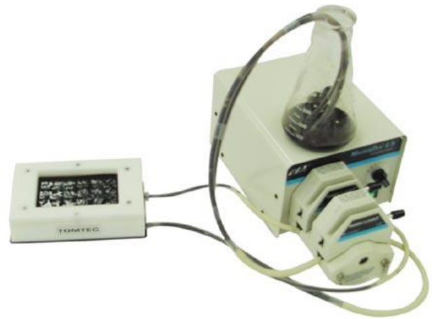
Figure 2. Live bottom recirculating constant level reservoir to maintain uniform magnetic particle suspension.
